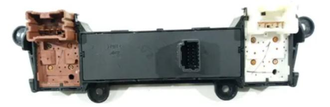
Install the one touch modules between the disconnected harness and its button. Installation is easy, just push the module's female connector into the button and the car harness female connector into module's male connector.
