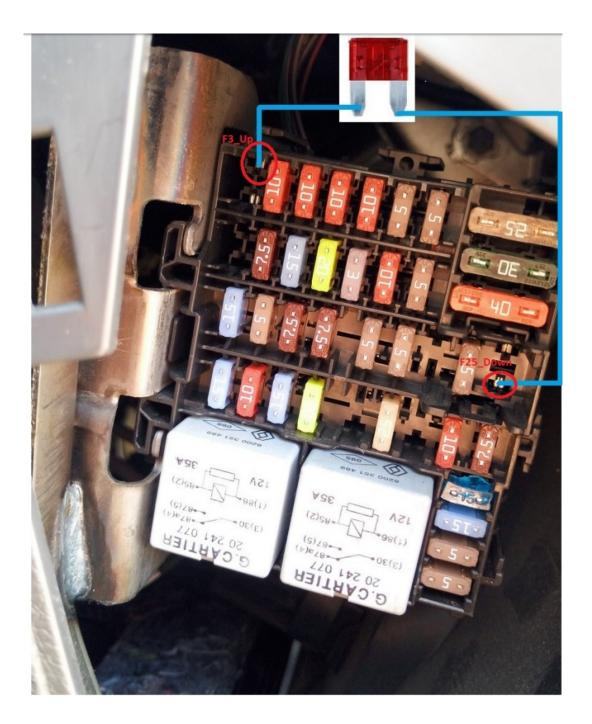
Now your electric window circuit is permanently powered no matter if Ignition is ON or OFF. Now test the function: exit the car and unlock it 3 times - windows should go down all the way. Lock the car 2 times - windows should go all the way up.
