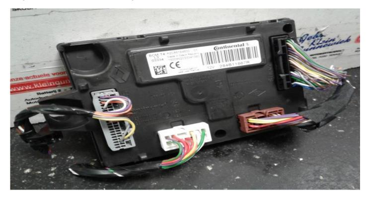
Now focus on the **Brown connector** which has the LOCK and UNLOCK signals to be wired to the one touch modules.
